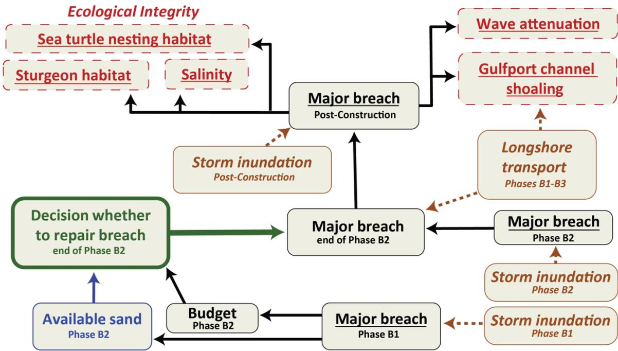
**Figure. 1** Influence diagram for decision model 1. External drivers (brown) are in italics with dashed arrows; decision node (green) is a thick box with thick arrow; and fundamental objectives (red) are in dashed boxes, a cluster of which are related to the ecological integrity of the beach and Mississippi Sound. Expert elicitation used for underlined nodes. The decision to repair a major breach in phase B1 is automatic, but influences the budget and available sand (in blue).
